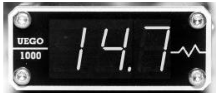
The display head above is showing an Air/Fuel ratio of 14.7:1, corresponding to a sensor driver voltage output of 2.57 volts.
